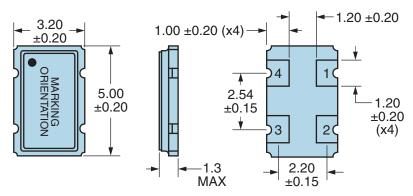
Note: Pin 1 Chamfer not shown.
